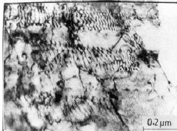
Fig. 2(a). Planar Dislocation arrangement, Microstructure A, Strain amplitude +0.4%
